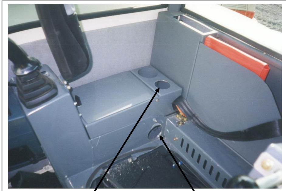
2 1/5" hole for snap-in louver
